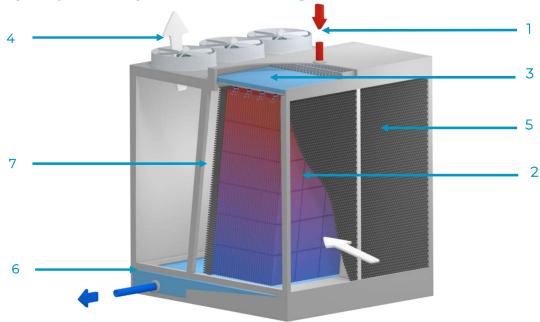
The hot water to be cooled is driven to the top of the device through pipes (1). This water is fractionated and distributed by gravity over the heat exchange surface (2) by low pressure water distribution nozzles (3).
